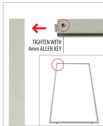
6. Attach horizontal frame sections
