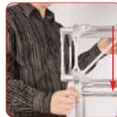
Align the arena section with the bolt holes on both sections
