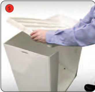
Take the shelf (C) and slide down through the top of the wrap.
