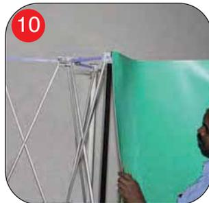
10-12. Hook graphic panel onto hookstuds and attach edge of panel to align with centre of magbar (on both edges of graphic panel). Attach remaining two panels similarly.
