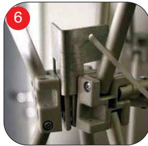
6-7. Insert attached aluminium brackets to two middle hubs to lock the frame in place.
