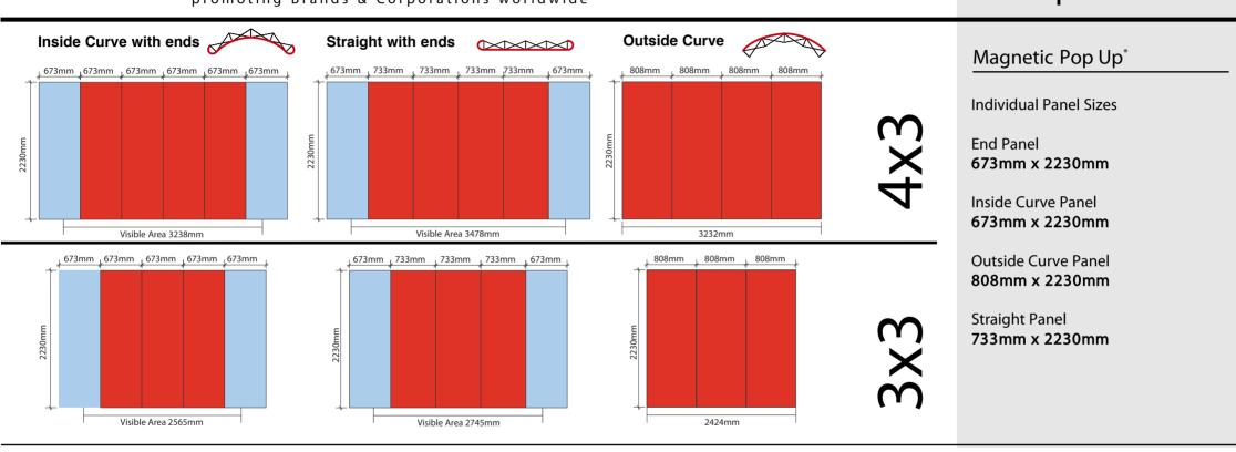
A stand is described by the number of frame squares wide (panels) x the number of frame squares high. Standard panel height of 2230mm increases to 2963mm for a 4-squares high frame, 3696mm for 5-squares high, and 4429mm for 6-squares high. Additional stabilising is recommended for increased heights, using either weights or our unique Frame Support Brace.
