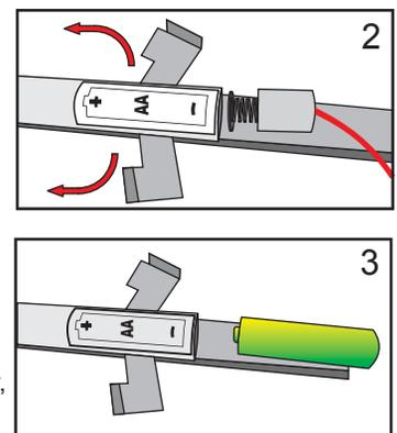
1. To replace the batteries , leave the Lantern collapsed. Grab the Lantern above the slider, around the fiberglass rods. Whilst holding the rods pull the fabric up the pole, exposing the two tubes that house the batteries.
