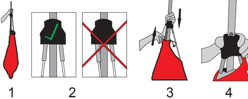
1. Remove the Lantern from the bag and place the Lantern upside down with the top cap on the floor.
