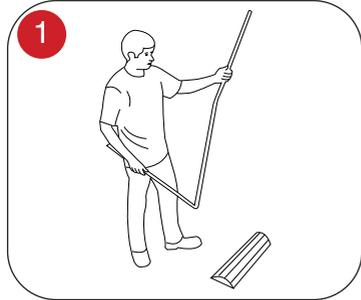
1. Assemble pole by connecting the attached sections together. Do NOT twist the pole sections once assembled as this can jam them together.
