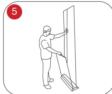
5. To display the second graphic, on a twin, stand facing the pole and pull out the second graphic from the base.
