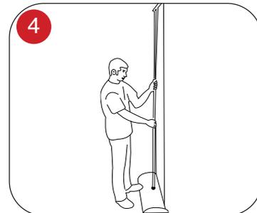
4. When the graphic and pole are fully extended and in an upright position, place the bottom of the pole in the centre hole of the base. Make sure it goes all the way down to the bottom of the hole. Then remove your foot from the base and wipe it clean please.
