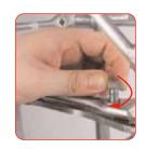
Slot the m8 bolt into the bolt hole
