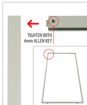
6. Attach horizontal frame sections
