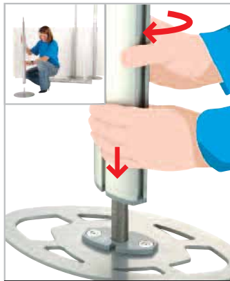
1. Twist'n'Lock male post onto base
