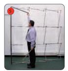
Add the mag bars onto the system, vertically for front and D-end panels. Then add horizontal mag bars across the top and bottom of the system.
