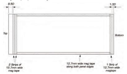
Apply mag tape to straight panels according to the diagram (all dimensions are approx).
