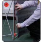
Smooth the graphic onto the mag bars, ensuring that it sits flat and is aligned to the centre line of each mag bar.
